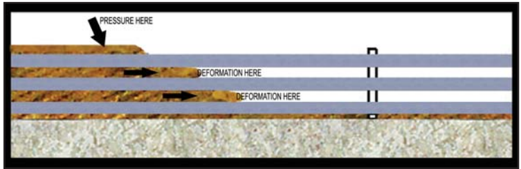
Figure 4. Illustrates the pressure applied to the native backfill area and the deformation that can occur in the transition area between native backfill and a slurry. In this transition area, proper compaction is difficult if not impossible to achieve. Without proper compaction the RHO values in these transition areas can be greatly increase, potentially causing overheating of the electrical conductors.
